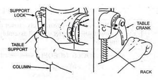
2. Remove protective covering from table and discard. Place table in table support and tinghten table lock (located under table) by hand.
