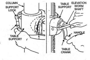
8. Check column collar for proper adjustment. Collar should not be angledon the column and it should be positioned so rack will slide freely in collar when table is rotated 360° around column table. If re - adjusted, only tighten set screw enough to keep collar in place.
