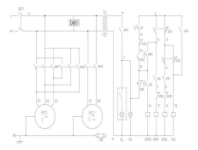
Wiring Diagram for 1 phase
