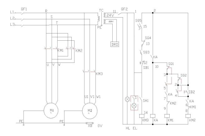
Wiring Diagram for 3 phases
