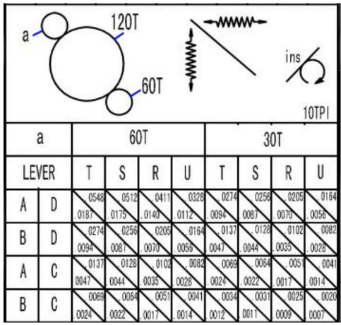
(b)Longitudinal and cross feed table for metric lathe
