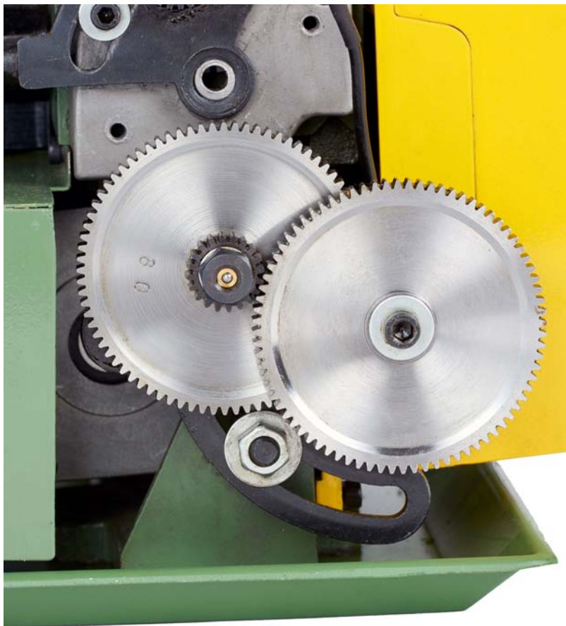
Figure 15 Change Wheel Gear Train - Shown Set for Fine Feed
