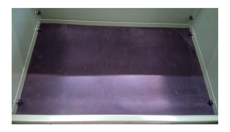
The stand is now complete you can now attach the tray and lathe to the stand using the large cap head bolts, Nuts, using the washers and sprung washers.
